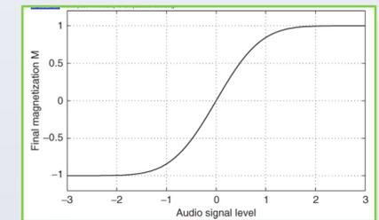
Fig. 5 – Typical Tape Saturation Curve (from [1])
