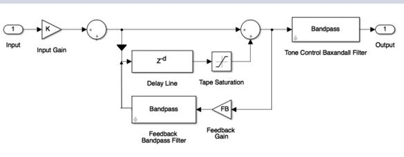
Fig. 1 – Signal Flow Diagram of Space Echo RE-201
