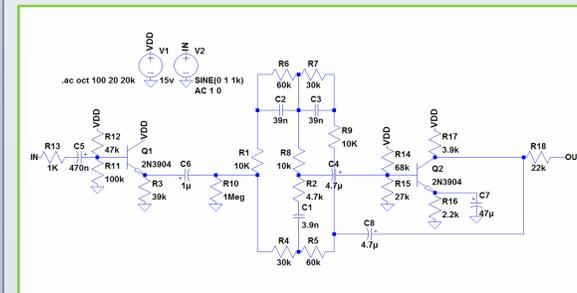
Fig. 3 – Filter Schematic for Roland Space Echo RE-201
