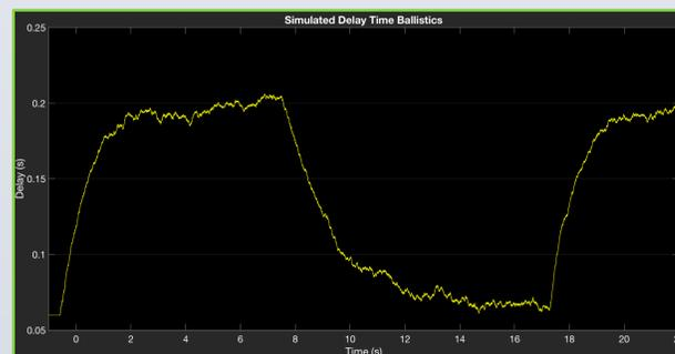
Fig. 2 – Simulated Delay Time Ballistics, Accounting for Wow and Flutter
