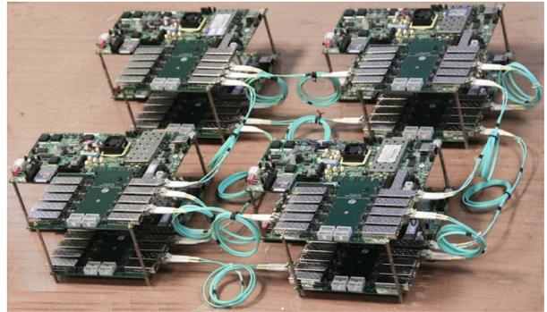
Figure 4: Eight-node prototype connected by a 3D-mesh network
