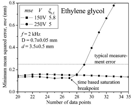
**Figure 10.** Plots of the mse calculated using eq A1 versus the number of experimental data points for data shown in Figure 6, based upon the best-fit coefficient values,  $\xi_{br}$ . At  $V = 150$  V-rms, which is below the saturation threshold, the mse remains constant as more points are added. On the other hand, at  $V = 250$  V-rms, above the saturation threshold, addition of the 28th data point, corresponding to  $t \sim 0.4$  s, heralds a rapid increase in the mse.
