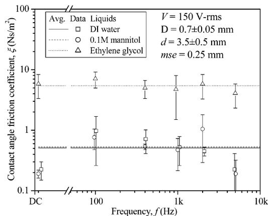
**Figure 8.** Plots of the coefficient  $\xi$  versus frequency for ethylene glycol and aqueous liquids showing at best modest dependence from dc up to 5 kHz. Note that the average value for ethylene glycol,  $\xi = 5.5$  (N s)/m<sup>2</sup>, is an order of magnitude higher than the value for aqueous solutions,  $\xi = 0.55$  (N s)/m<sup>2</sup>.
