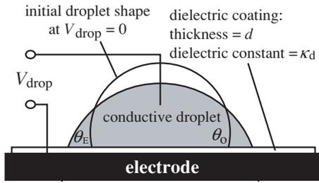
**Figure 1.** Electrowetting behavior of a sessile droplet of conductive liquid on a dielectric-coated electrode. An applied voltage between the droplet and the electrode caused the droplet to spread on the substrate.
