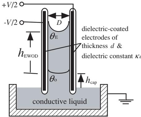
**Figure 2.** Height-of-rise experiment with coated electrodes and conductive liquid. Application of voltage lifts the liquid column upward between the parallel electrodes and reduces the apparent contact angle.
