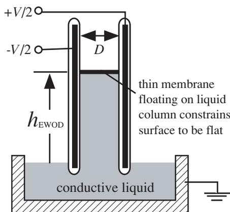
**Figure 3.** Thought experiment with the top surface of the liquid column between parallel electrodes constrained by a very thin, rigid, electrically insulating membrane that slides up and down without friction. The meniscus remains flat as the column rises in response to increasing the voltage.
