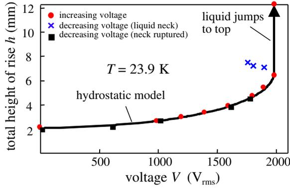
**Figure 10.** Experimental data and predicted  $h(V)$  curve from equation (6) for converging plates,  $w = 7.6$  mm,  $H = 12$  mm,  $a = 0.42$   $\mu\text{m}$ ,  $b = 1.41$   $\mu\text{m}$ . The data obtained for increasing voltage (●) match the prediction very well. For decreasing voltage, data indicated by (×) indicate the location along the vertical sides where the interface is collapsed inwards the most. The squares (■) denote the height of the column after the neck has ruptured.
