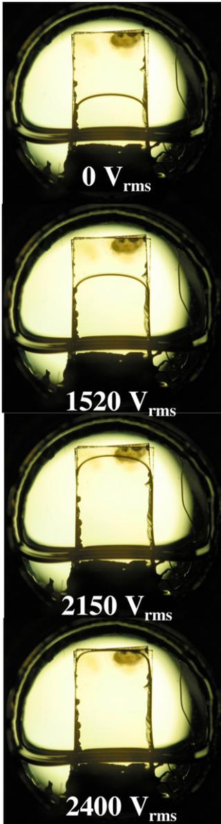
**Figure 2.** Meniscus of cryogenic  $D_2$  at  $T = 18.7$  K viewed through parallel, transparent ITO-coated glass electrodes,  $w = 7.6$  mm,  $d = 0.86 \mu\text{m}$  for 1 kHz ac voltages ranging from 0 to  $2400 V_{\text{rms}}$ . Frequency must be high enough to avoid surface wave instabilities, but is otherwise not important.
