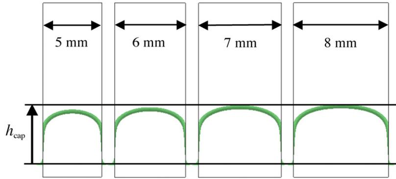
**Figure 6.** Side view of liquid  $D_2$  meniscus profile between plates of spacing  $d = 0.86$  mm at  $T = 18.7$  K calculated using *Surface Evolver* for different values of the plate width:  $w = 5, 6, 7$  and  $8$  mm. The top of the liquid column does not reach  $h_{\text{cap}}$ , the value predicted by the one-dimensional model, equation (1), unless  $w \geq 7$  mm. This result may be expected to scale directly with plate spacing  $d$ .
