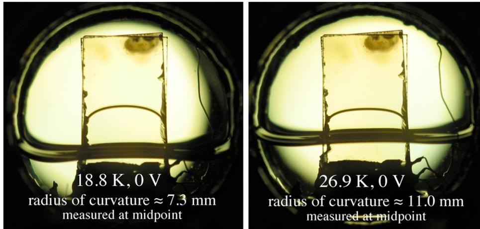
**Figure 4.** Effect of temperature on meniscus shape and height-of-rise  $h_{\text{cap}}$ . The temperature, but not the electric field  $E$ , affects the profile of the meniscus along the width of the electrodes through its influence on surface tension and density.
