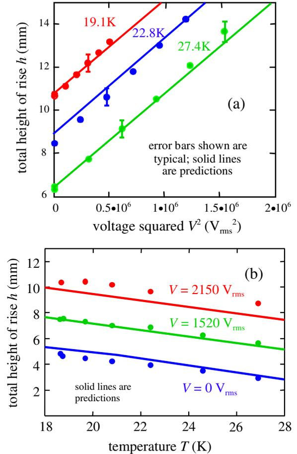
**Figure 3.** Height-of-rise data and predictions using  $h(V) = h_{\text{cap}} + h_{\text{DEP}}(V)$  for liquid deuterium using parallel electrodes:  $w = 7.6$  mm,  $d = 0.43(\pm 0.02)$  mm. (a)  $h$  versus voltage  $V$  at various temperatures. (b)  $h$  versus temperature at several fixed voltages.
