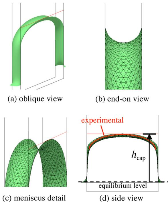
**Figure 5.** Numerical solution obtained using *Surface Evolver* software for the shape of the liquid meniscus between parallel plates for  $w = 7.6$  mm,  $d = 0.86$  mm and  $T = 18.7$  K. (a) Oblique view. (b) End-on view showing the contact angle  $\theta_c \approx 0^\circ$ . (c) Close-up of the meniscus. (d) Side view, perpendicular to parallel plates, with superimposed profile obtained from experiment.  $h_{\text{cap}}$  is the height of rise calculated from equation (1).
