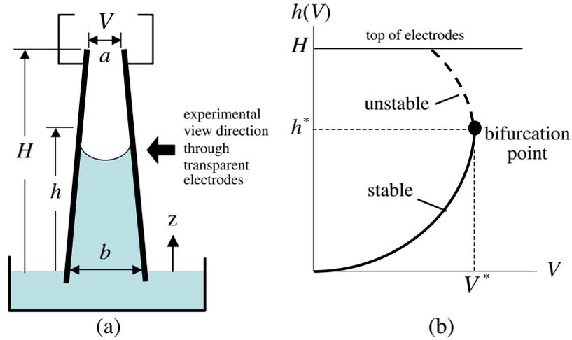
**Figure 7.** The converging plate experiment. (a) Side view of electrode geometry with definitions of parameters. (b) Representative  $h(V)$  curve with bifurcation point at  $(V^*, h^*)$ . Bifurcation is experimentally observable only if the electrode height  $H$  exceeds the critical value, that is  $H > h^*$ .
