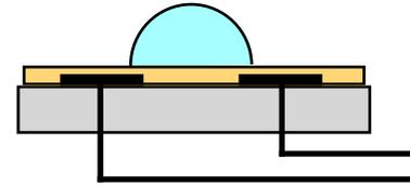
Fig. 1. Basic coplanar structure of electrodes forms a non-uniform E field that creates new hydrostatic liquid equilibrium with semicircular cross-section. Raising voltage increases both semicircular radius and max. flow rate.
