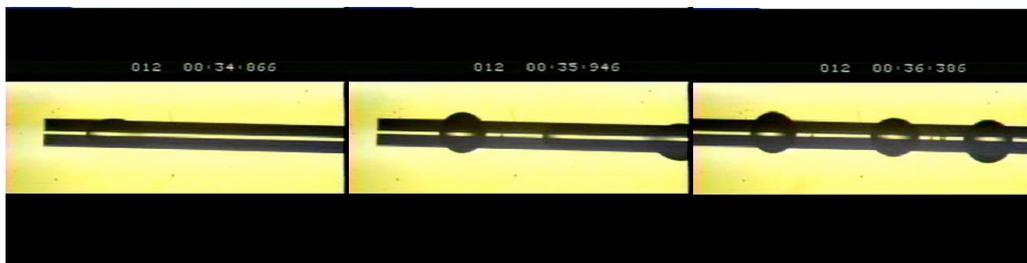
Fig. 4. Selected video frames showing capillary induced break-up of liquid finger into droplets. Near the end of the structure, surface tension simultaneously draws the finger from left to right back to the liquid reservoir, but instability proceeds more quickly.
