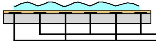
Fig. 3. Cross-section of liquid film created by array of parallel electrode strips.
