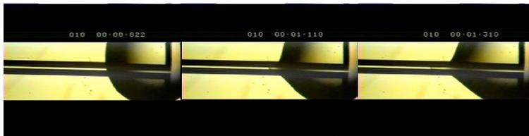
Fig. 2. Selected video frames of liquid motion immediately after applying voltage. Starting from the liquid reservoir at right, the finger travels to the left. The liquid is 50 cS silicone oil. Electrode width = 90  $\mu\text{m}$ ; gap = 30  $\mu\text{m}$ ; voltage = 625 V-rms; frequency = 100 Hz.
