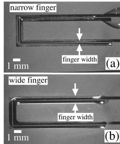
FIG. 8. Indeterminacy of liquid configuration for coplanar electrodes: width  $w = 500 \mu\text{m}$ ; gap spacing  $g = 100 \mu\text{m}$ ; polyimide layer  $t = 10 \mu\text{m}$ . Both experiments conducted at  $V_s \sim 700$  V and  $f = 100$  kHz. (a) Narrow water finger confined to vicinity of gap; (b) wide water finger spanning entire width of electrode structure.
