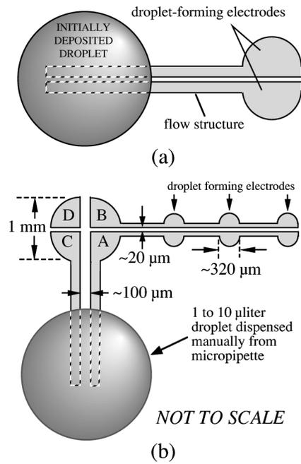
FIG. 6. Coplanar electrode configurations for droplet formation (not shown to scale). (a) Basic structure for droplet formation using bisected circular electrodes; (b) two-stage droplet formation structure. To fill intermediate reservoir from large droplet, electrodes A and B are connected together, as are C and D. After the reservoir is filled, A is connected to C and B is connected to D for droplet formation.
