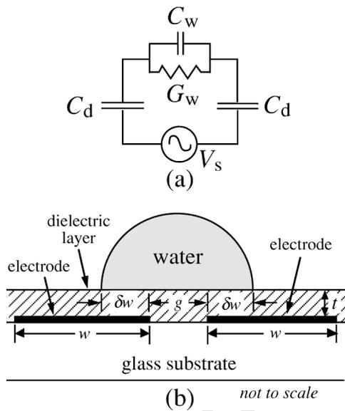
FIG. 5. Circuit model and cross section of flow structure. At high frequency (i.e.,  $f \gg f_c$ ), voltage drops across the bulk of the water, thus establishing the strong, nonuniform electric field that collects liquid in compact semicircular profile. (a) RC circuit model for the DEP actuator. (b) Semicircular cross section of liquid-filled flow structure for computation of circuit parameters. Sketch is not to scale.
