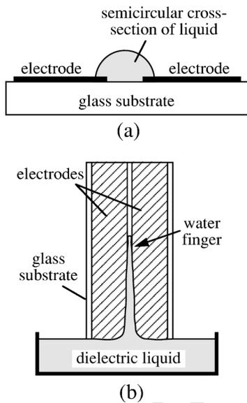
FIG. 2. Planar electrode configurations for wall-less flow structures. Sketches are not to scale. (a) Cross section of original microelectrode structure used with insulating transformer oil. The liquid forms a semicircular profile centered on the gap. (b) Side view of dielectric height-of-rise experiment showing liquid finger extending upward in the gap between the coplanar electrodes.
