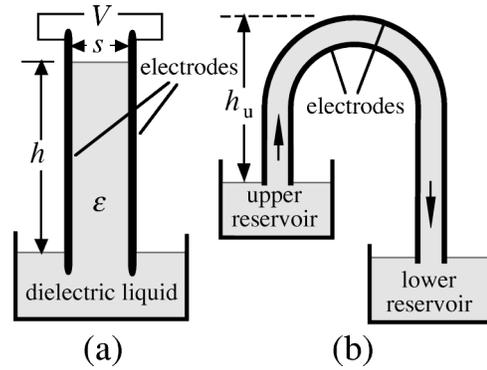
FIG. 1. Dielectrophoresis of insulating dielectric liquids. (a) Pellat's original experiment (Ref. 19). (b) The dielectric siphon experiment (Ref. 20).
