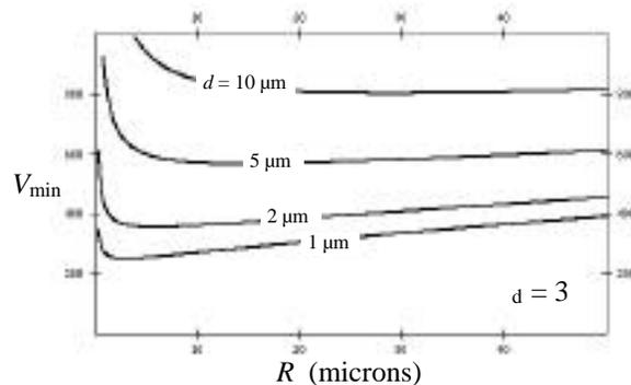
Fig. 2 Minimum voltage for DEP actuation,  $V_{\min}$  from Eq. (12), plotted versus finger radius  $R$ , with  $g = w = 2R/3$  for  $d = 1, 2, 5, \text{ and } 10 \mu\text{m}$ .
