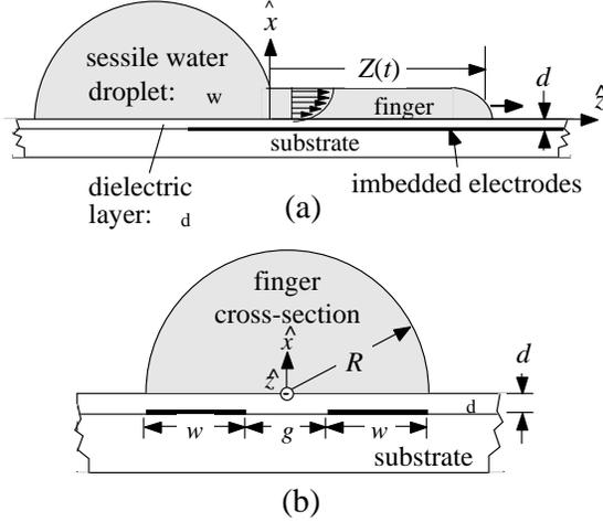
Fig. 1 Simple model for water finger extending from a large droplet. (a) Side view with definitions for  $Z(t)$  and other quantities. (b) Semi-circular cross-section of finger of radius  $R$  and substrate showing location of electrodes and dielectric layer of thickness  $d$  and dielectric constant  $\epsilon_d$ .
