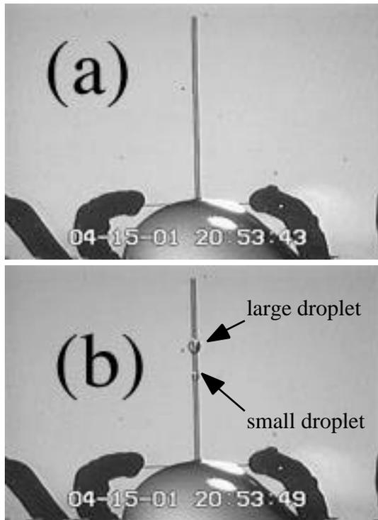
Fig. 7 Micrographs from videotape of droplet formation with de-ionized water using a straight electrode structure of length  $2000 \mu\text{m}$ :  $d = 10 \mu\text{m}$ ,  $w = 20 \mu\text{m}$ .  $g = 20 \mu\text{m}$ . a) Before removal of voltage; b) after removal of voltage. Two droplets of estimated volumes  $\sim 820$  and  $\sim 93$  picoliters are visible. Most of the water has been drawn back into parent drop visible at bottom of image.
