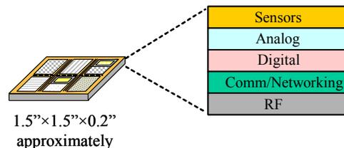
HSoC: four types of sensors (acoustic, seismic, visible spectrum and IR imaging), decision capability, and *ad hoc* networking. Not shown is the package.
