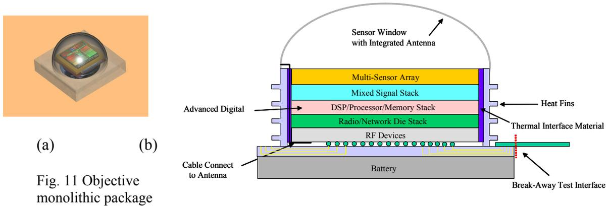
Fig. 11 Objective monolithic package
