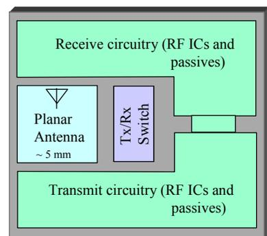
Fig. 9 RF plane (an outer plane)
