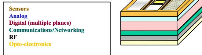
**Fig. 2 3D Heterogeneous System on a Chip**
