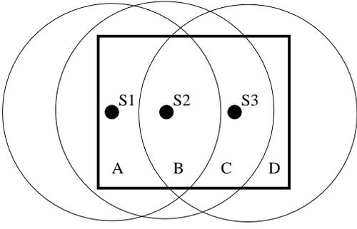
Fig. 2. Example sensor network. Since  $s_3$  is the only sensor that can cover region D, its worst coverage-based cost  $C_{wc}(s_i)$  is the highest in the network. The comprehensive coverage-based cost  $C_{cc}(s_i)$  gives a more complete encapsulation of a sensor's value to the sensing task and considers the area and redundant energy of each subregion.
