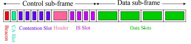
Figure 2. MH-TRACE frame structure.
