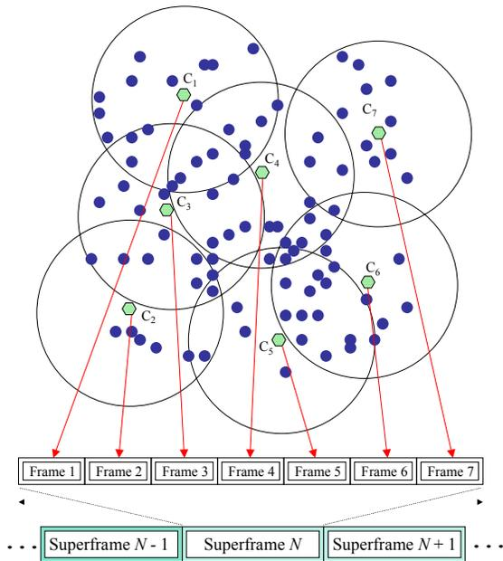
Figure 1. A snapshot of MH-TRACE clustering and medium access for a portion of an actual distribution of mobile nodes. Nodes  $C_1 - C_7$  are CHs.
