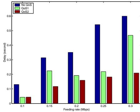
**Figure 2.** Real-time data flow's average packet delay.
