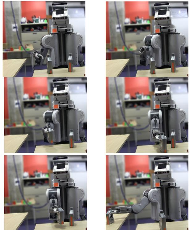
Fig. 1: Actions in response to the goal of having a heavy oil bottle on the table to the right. The robot picks up one bottle, feels that it is light, picks up the other one, and places it on the correct table, requiring re-planning and sensing.
