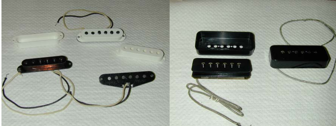
Figure 1: Left – Fender Stratocaster Pickups; Right – Gibson P-90 Pickups
