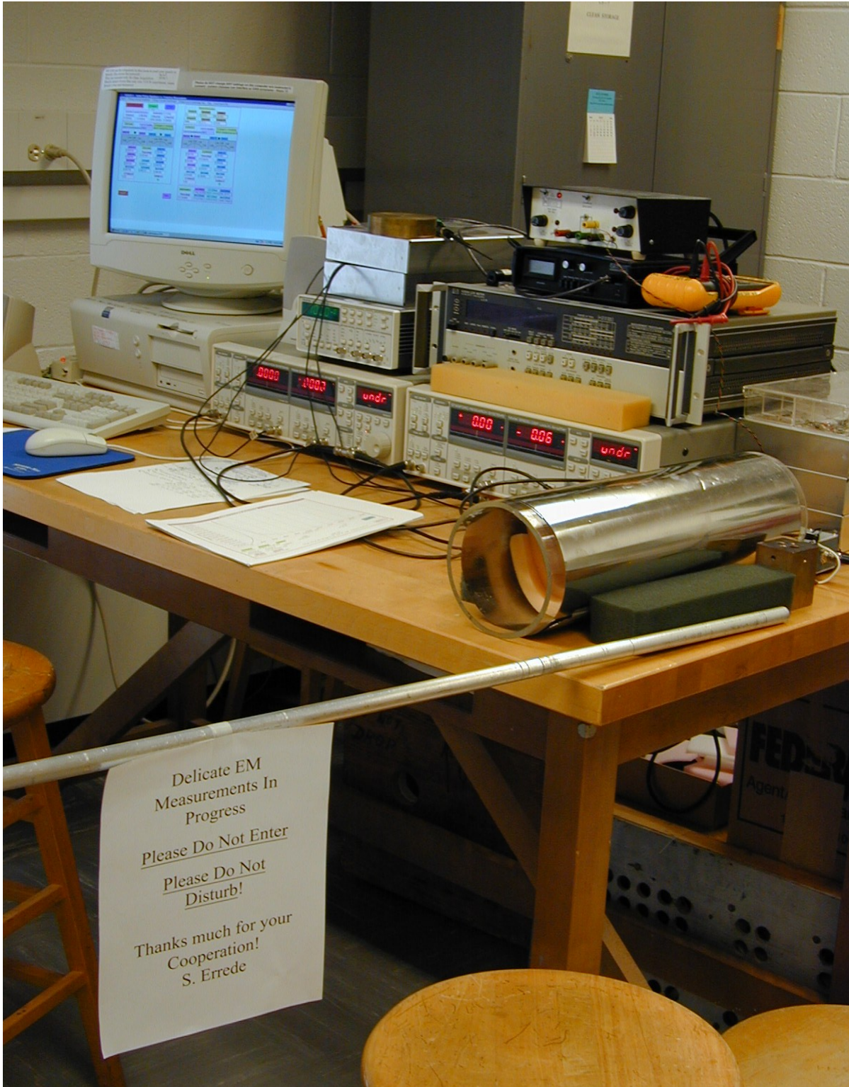
Figure 2: UIUC Physics 498POM Electric Guitar Pickup Measurement Facility
